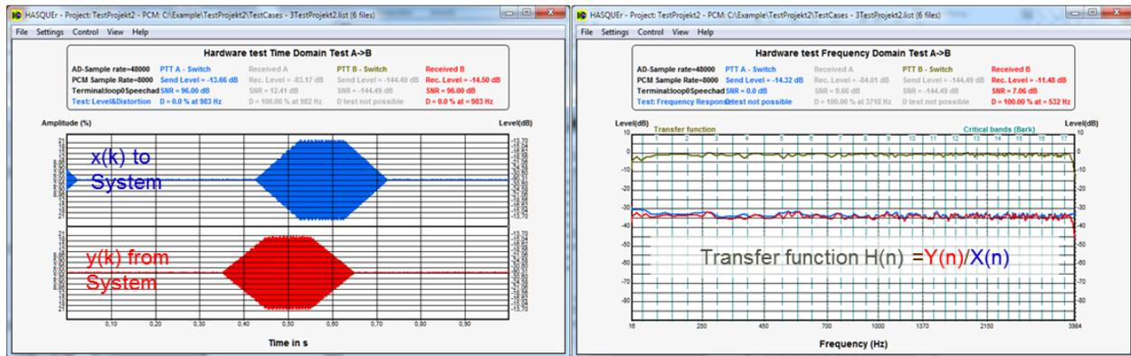
Figure 4: Function test of the connected system under test by simple mouse click
