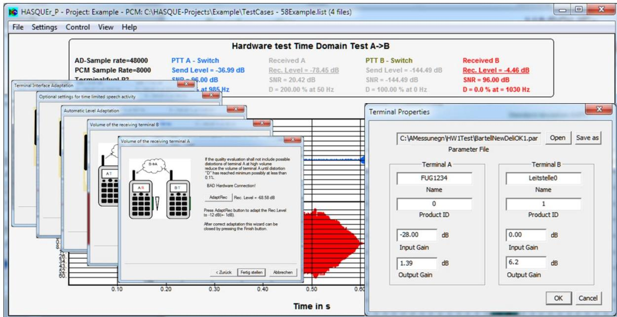
Figure 5: Automatic level adaptation between measurement system and system under test
