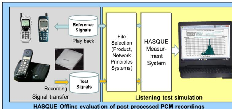
Figure 7: Offline measurement system
